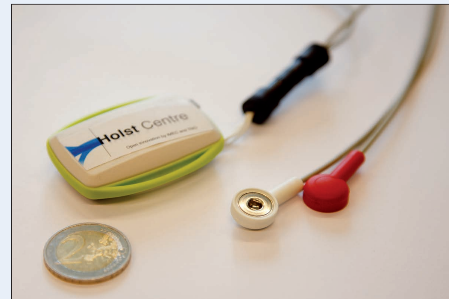
Figure 1 Prototype wearable system for real-time heart rate based seizure detection.
